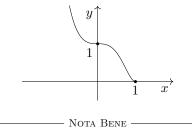
Having removed points from the graph, the SP at (0, 1) is only a one-sided minimum. This doesn't, in the final graph, distinguish it from a point of inflection. But the classification is still relevant to the sketch, as it distinguishes between a minimum and a maximum.
